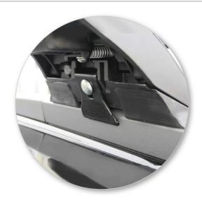
Ensure the clamp engages correctly in slot inside of roof rail.
