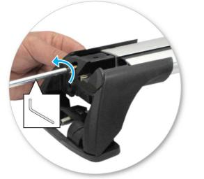
Use hex screwdriver to reverse adjusting screw 10 turns.
