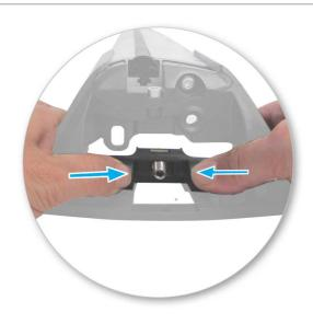
Remove plastic clamp block by gripping bar leg with fingers and push firmly with thumbs until clamp block drops out behind leg.
