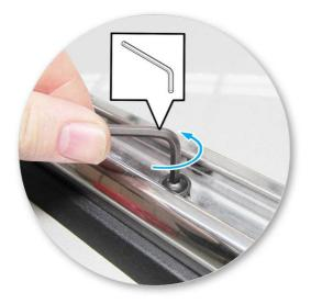
Remove screws from the vehicle's fixed points
