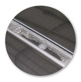
Remove rubber washer from screw and reinstall onto fixed point.
