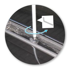
Remove screws from the vehicle's fixed points
