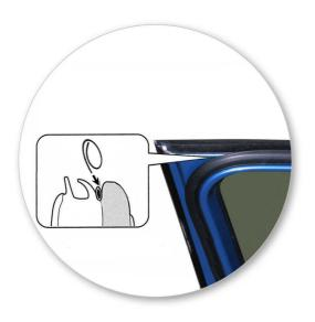
• Ensure door seal positioned as shown.
