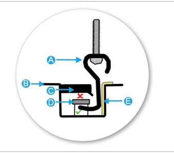
A= Clamp B= Roof line C= Body trim D= Vehicle fixpoint E= Protective strip
