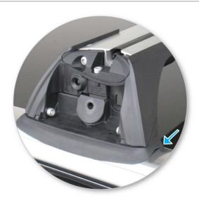
Ensure back edge of foot sits flush with the back edge of vehicle roof rail.
