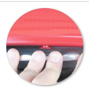
The rubber seal must be peeled back from the vehicle body to allow the clamp to be inserted between the vehicle body and the rubber seal.
