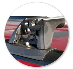
• Ensure that the cover plate and foot sit firmly on the roof.
