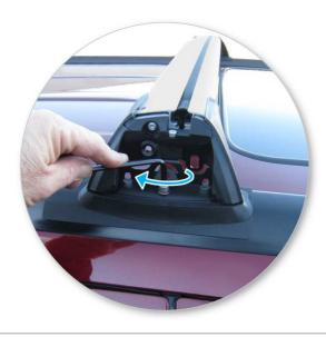
Tighten foot and cover plate down using the Hex Key.
