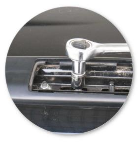
The fixed point studs have a thick layer of paint. Remove paint by using the M8 nut supplied. Use a socket spanner and run the nut down the centre stud only.
