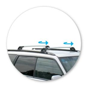
Place crossbars back onto vehicle roof by placing one end of crossbar on the rail and swing the other into previously marked position.
