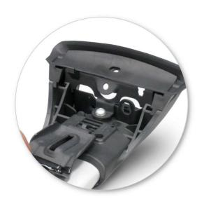
Remove crossbar off vehicle and turn upside down. Select metal clamp and fit small tongue into position 2 marked on the leg.
