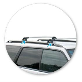
Temporarily mark with masking tape or pencil the position of crossbars on the rail.
