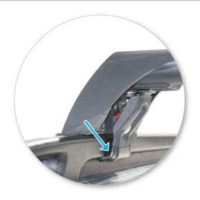
Ensure the clamp engages correctly on inside of roof rail.
