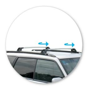
Place crossbars on vehicle roof by placing one end of crossbar on the rail and swing the other crossbar into position.
