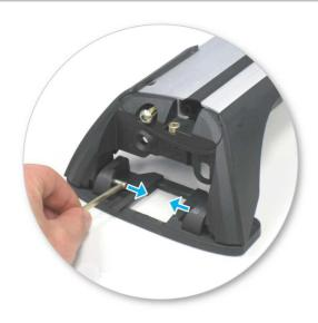
Remove both pins from each leg. Use tapered end of spanner located inside left hand cover to assist.
