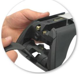
Attach clamp to each leg. NOTE; clamps may have labels showing their positions on the vehicle (For example; "Front Right").
