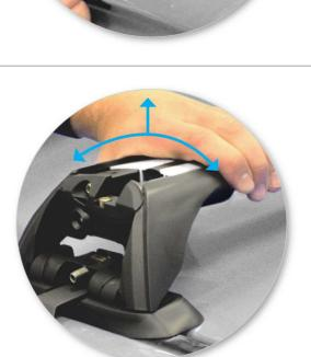
• Check crossbar is securely attached to the vehicle.
