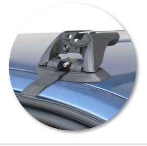
Clamps under rubber door frame mouldings
